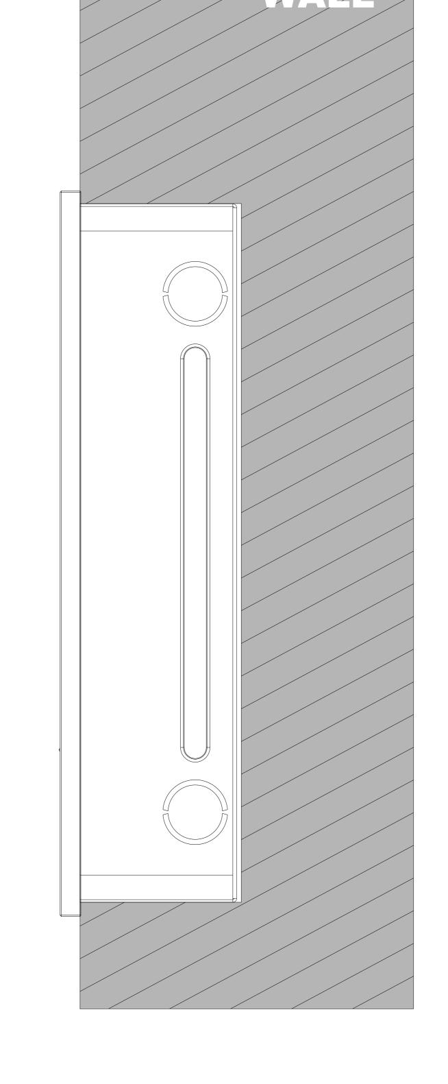
**FRONT VIEW: FLUSHING MOUNTING BOX PLACEMENT**
