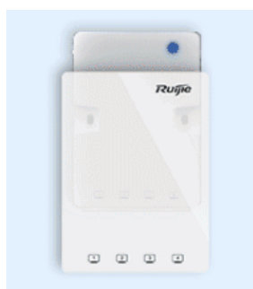
Device Status Lighting is covered by plate
